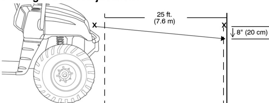
1. Place the vehicle on a level surface with the headlight approximately 25 ft. (7.6 m) from a wall.
