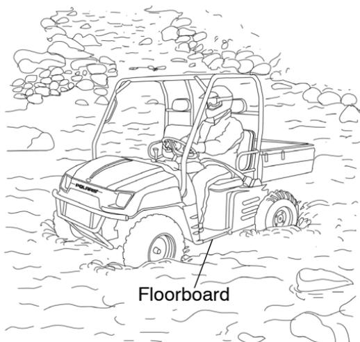
**NOTE:** After running your vehicle in water, it's *critical* that you perform the services outlined in the Periodic Maintenance Chart beginning on page 58. Give special attention to engine oil, transmission oil, front and rear gearcases, and all grease fittings.
