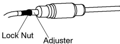
**NOTE:** While adjusting, lightly flip the throttle pedal up and down.
