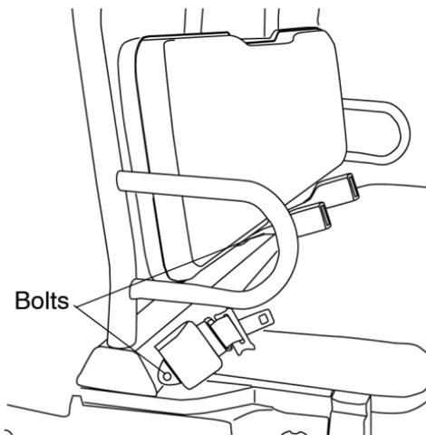
1. To adjust, loosen the bolts.
