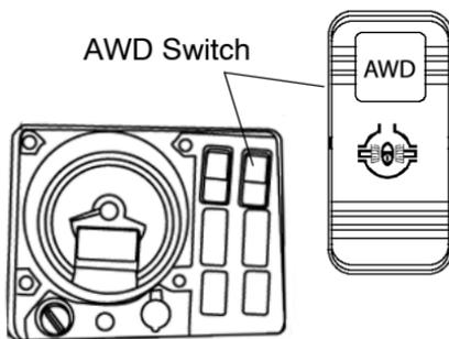
When the *RANGER* 6X6 AWD switch is in the off position, the vehicle is in two-wheel drive at all times.
