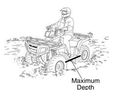
NOTICE: Major engine damage can result if the vehicle is not thoroughly inspected after operation in water. Perform the services outlined in the maintenance chart. See page 62. The following areas need special attention: engine oil, transmission oil, demand drive fluid, rear gearcase oil, and all grease fittings.
