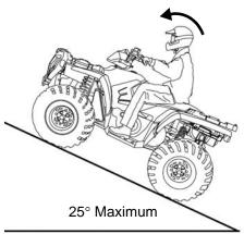
Braking and handling are greatly affected when operating in hilly terrain. Improper procedure could cause loss of control or overturn. Whenever traveling uphill, follow these precautions:
