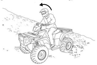
Driving on a sidehill is not recommended. Improper procedure could cause loss of control or overturn. Avoid crossing the side of any hill unless absolutely necessary.
