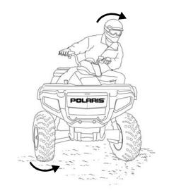
of traction between the rear wheels, allowing the turn to be made smoothly. The same leaning technique should be used for turning in reverse.
