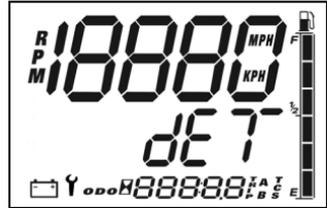
If *severe* detonation occurs, the check engine light will begin to flash steadily and the gauge indicator will read “DET” (see illustration). The engine will enter a *limp home* mode and RPM will be limited to 6500 RPM. The engine will remain in this mode until it is shut down and restarted.
