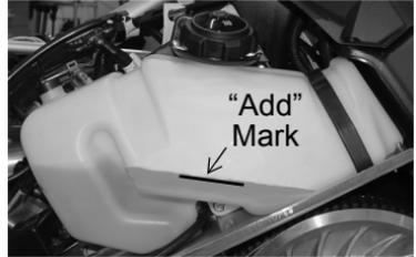
**NOTICE:** Operating the snowmobile without adequate engine lubrication can result in serious engine damage. Always check the oil level when refueling. Add oil as needed.
