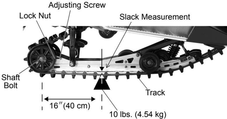
8. Tighten or loosen the track adjusting screws to provide equal adjustment on both sides of the track.
