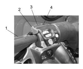
**TIP:** If the brake lever is squeezed tightly enough, the lock will move freely into place. Do not force the lock or it may break.
