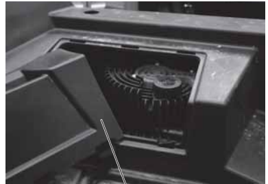
Oil Tank Access Panel
