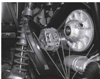
Remove ALL Debris
