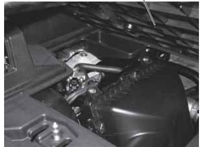
Cargo Box Access Panel
