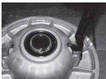
Insert hooked end of tool.
