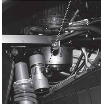
Oil Tank Drain Plug
