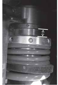
Walker Evans Rear Shock Preload Measurement
