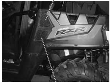
PVT Intake Pre-Filter
