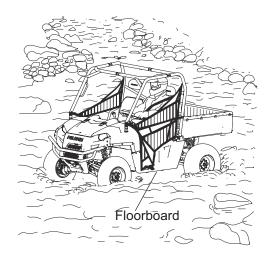
**NOTICE:** After running your vehicle in water, it's critical that you perform the services outlined in the Periodic Maintenance Chart beginning on page 43. Give special attention to engine oil, transmission oil, all gearcase fluids, and all grease fittings.
