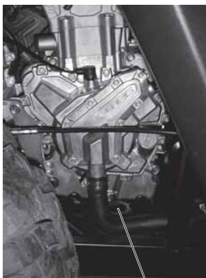
Drain Plug Access
