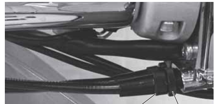
Adjuster Nut Lock Nut
