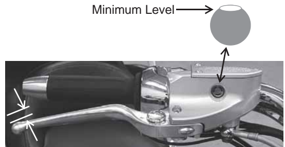
Resistance at 3/4 inch (19 mm)
