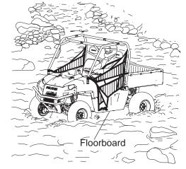
After leaving water, always dry the brakes by applying light pressure to the pedal repeatedly until braking action is normal.
