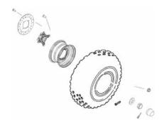
**WARNING!** Improperly installed wheels can adversely affect tire wear and vehicle handling, which can result in serious injury or death. Always ensure that all nuts are torqued to specification. Do not service axle nuts that have a cotter pin installed. See your POLARIS dealer.
