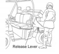
**WARNING!** If the weight distribution on the box is located toward the rear of the box when the release lever is pulled forward, the box may dump unexpectedly and cause serious injury to the operator or bystanders. Never operate the dump lever without ensuring that the load is positioned evenly or at the front of the box.
