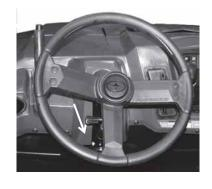
If the vehicle is in any gear other than neutral with the park brake engaged, "BRAKE" flashes in the rider information display. If throttle is applied and engine speed reaches 1200 RPM, an alarm will sound to alert the operator.
