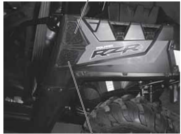
PVT Intake Pre-Filter
