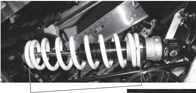
Installed Length Measurement
