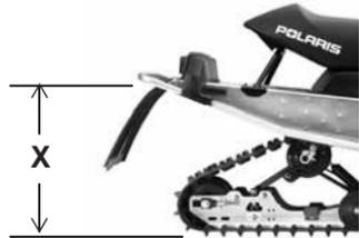
Next, have the rider drop down hard on the seat and bounce up and down several times, collapsing the rear suspension. With the rider seated, measure the distance between the ground and the rear bumper at the exact location used for measurement X. This is measurement Y.
