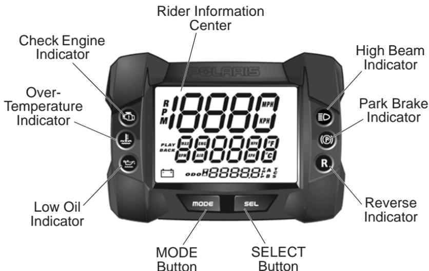
The instrument cluster contains indicator lights and the rider information center. The information center can be controlled by either the MODE and SELECT buttons on the instrument cluster or by the MODE/SET switch on the left handlebar.
