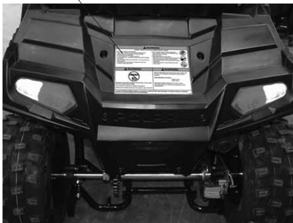
Rear Warning Label
