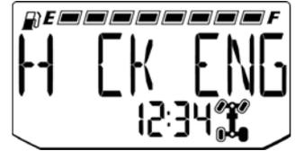
1. If the trouble codes are not displayed, use the MODE button to toggle until “CHK ENG” displays on the information display area.
