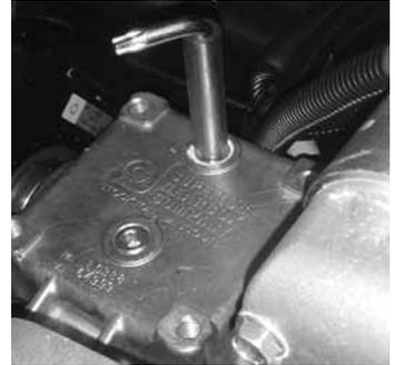
9. If the breather tube has been allowed to hang down, water can enter the breather tube and be sucked into the gearcase.
