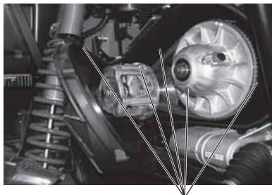
Remove ALL Debris
