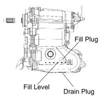
Access the transmission fill plug from the right side of the vehicle. Access the drain plug from the left side of the vehicle.
