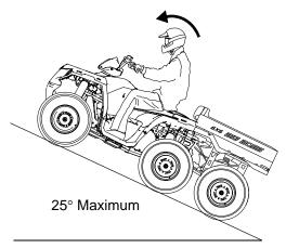
Braking and handling are greatly affected when operating in hilly terrain. Improper procedure could cause loss of control or overturn. Whenever traveling uphill, follow these precautions:
