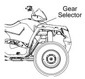
**NOTICE:** Shifting gears with the engine speed above idle or while the vehicle is moving could cause transmission damage.
