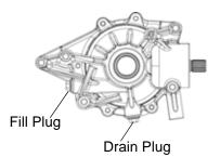
We recommend the use of POLARIS ATV Angle Drive Fluid (or GL5 80-90 weight gear lube). See page 124 for the part numbers of POLARIS products.
