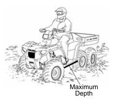
**NOTICE:** Major engine damage can result if the vehicle is not thoroughly inspected after operation in water. Perform the services outlined in the maintenance chart. See page 67. The following areas need special attention: engine oil, transmission oil, demand drive fluid, rear gearcase oil, and all grease fittings.
