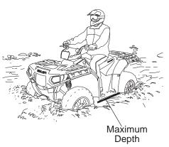
**NOTICE:** Major engine damage can result if the vehicle is not thoroughly inspected after operation in water. Perform the services outlined in the maintenance chart. See page 85. The following areas need special attention: engine oil, transmission oil, demand drive fluid, rear gearcase oil, ADC fluid and all grease fittings.
