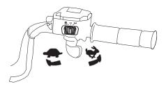
open position when the operator releases the throttle lever, engine speed will be limited, and power to the rear wheels will be reduced.
