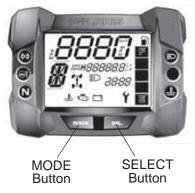
quickly. The transmission cannot be in reverse when using the override button as a MODE or SELECT button. This feature does not contain a vehicle speed lockout function and can be used at any operating speed.
