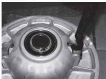
Insert hooked end of tool.
