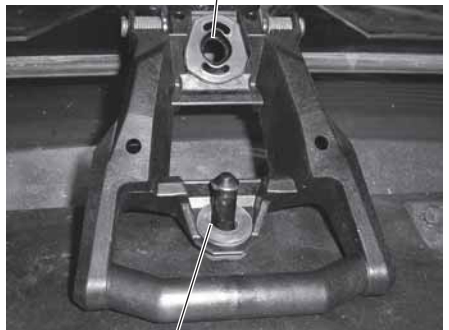
Rear Ring (secures a vented windshield)
